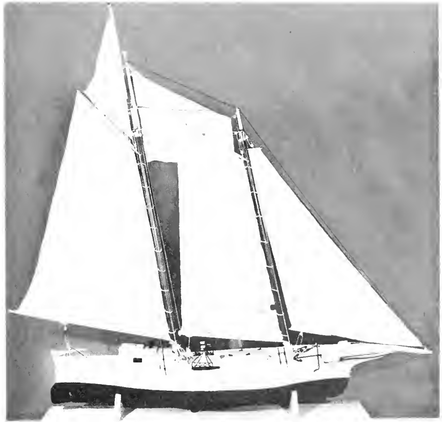
SCHOONER - RIGGED CHESAPEAKE BAY BUGEYE, 1865-75, referred to locally as "square-rigged." Rigged model USNM 42757. (Smithsonian photo 45605-f.)
